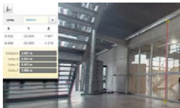
Site awareness and visualization - remotely checking the size and shape of a building
