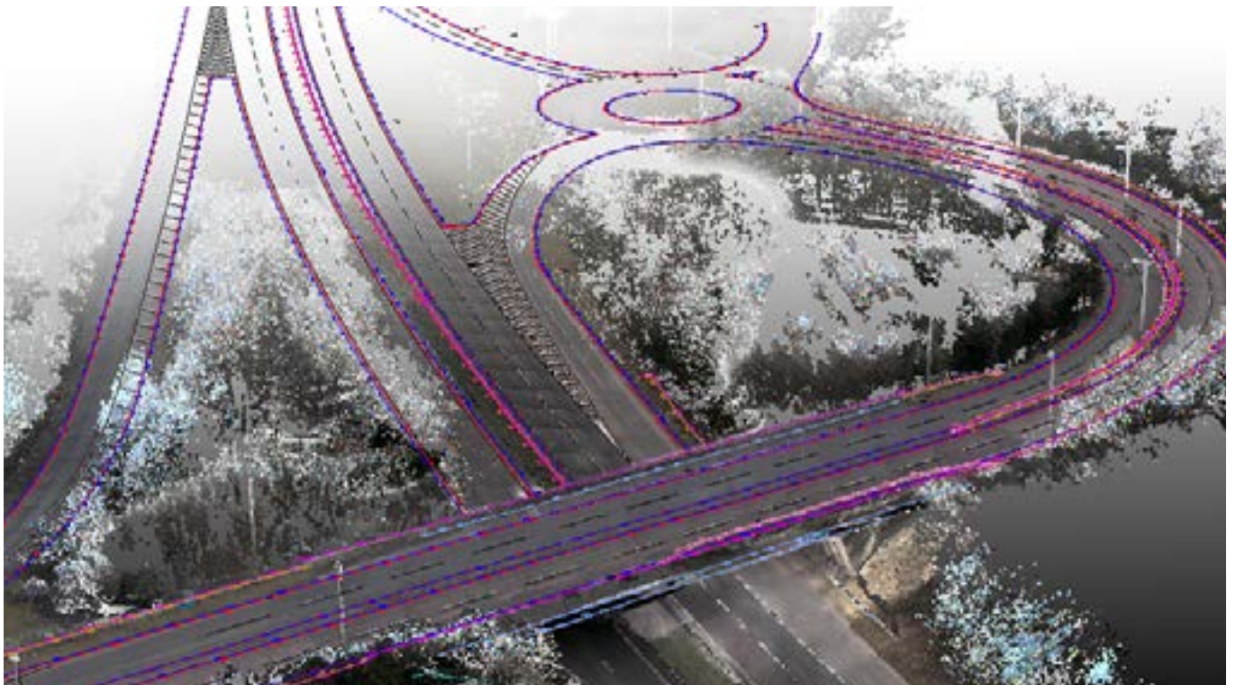
Application of reality capture - mobile mapping of existing road
