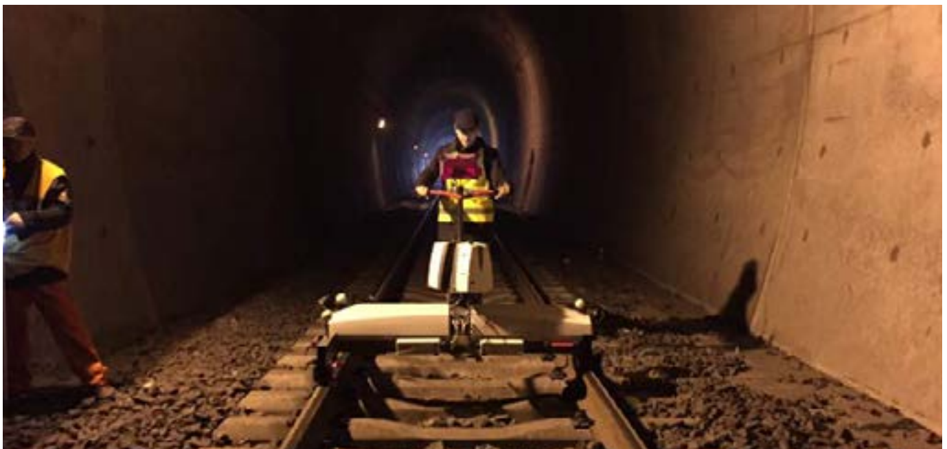
Application of reality capture - capturing existing rail track
