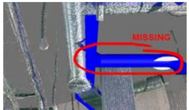
Construction verification - spotting irregularities to the structural steel frame
