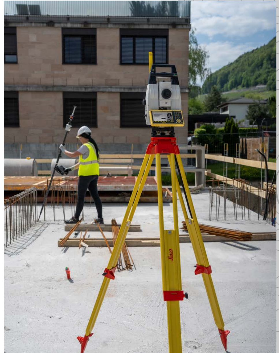
Robotic total stations combined with innovations such as the Leica AP20 AutoPole smart prism pole system provide significant time savings for layout. Learn more.
